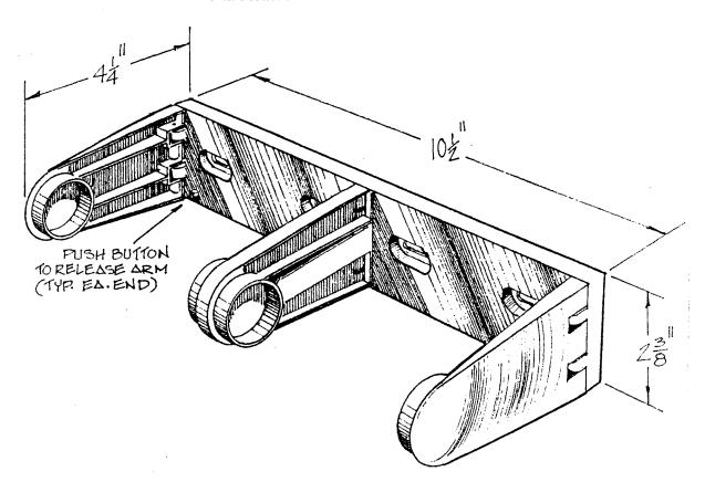
CONSTRUCTION: Double Roll Toilet Paper Holder is fabricated of die cast polished zamak,
