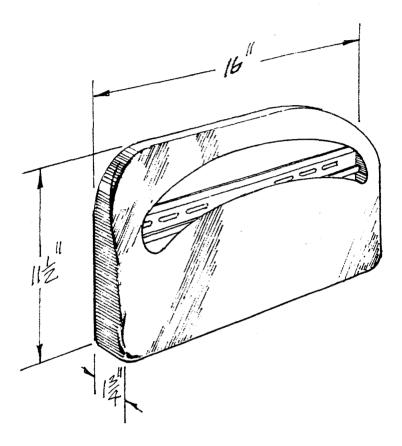
**CONSTRUCTION:** The CW45C is fabricated of chrome plated steel.
