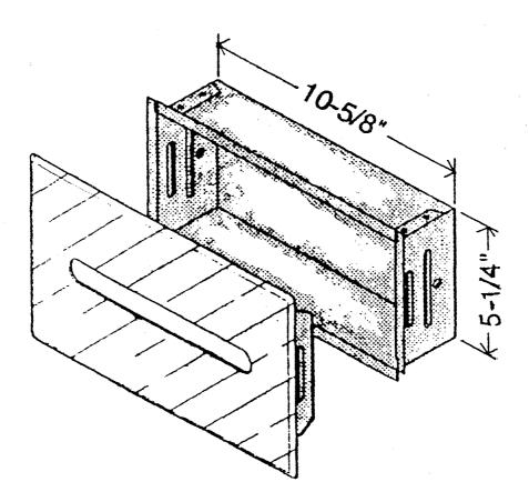
CONSTRUCTION: FACEPLATE FABRICATED OF STAINLESS STEEL.
