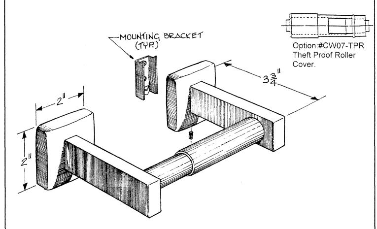
**CONSTRUCTION:** END BRACKETS are type 304 brite stainless steel.
