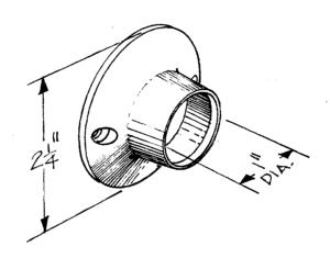
CONSTRUCTION: The #103 shower rod flange is chrome plated die-cast
